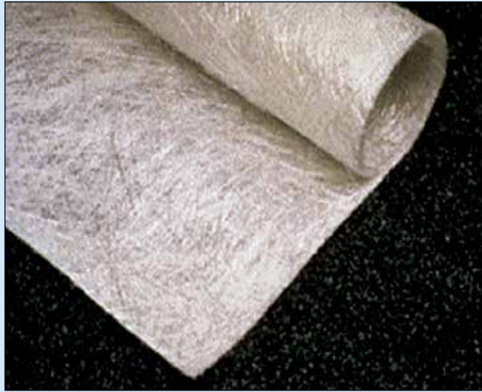
FIGURE D.4-2: Randomly oriented fibers shown in a roll of chopped strand mat
