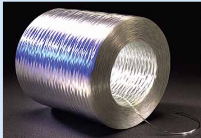
FIGURE D.4-3: Single-end roving for pultrusion
