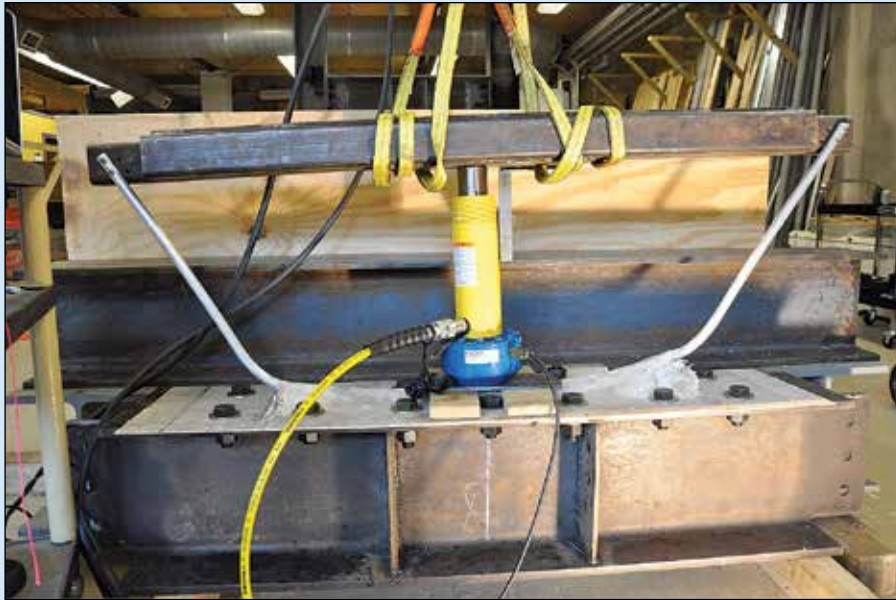
FIGURE L.6: Connection capacity testing – aluminum rod to FRP laminate
