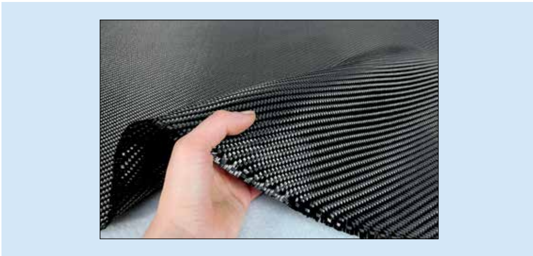
FIGURE D.4-4: Carbon-fiber-woven roving ply, with fibers in two orthogonal directions, [0/90] to the sheet direction
