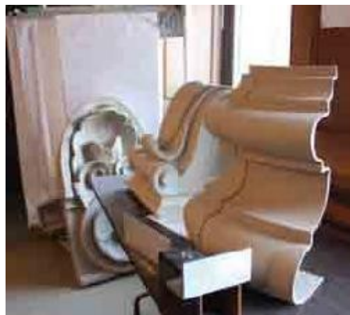
MATERIAL IMPROVEMENTS Fiberglass cornices and other shapes, supplied by Architectural Fiberglass Inc., were used to replace damaged terra cotta.
