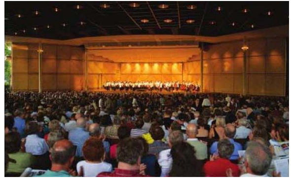
Acoustically reflective FRP walls at Chicago Symphony's Ravinia Festival Outdoor Pavilion in Illinois.
